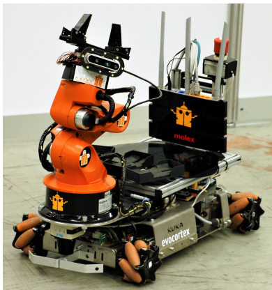
Fig. 2: KUKA youBot platform of the team AutonOHM.
