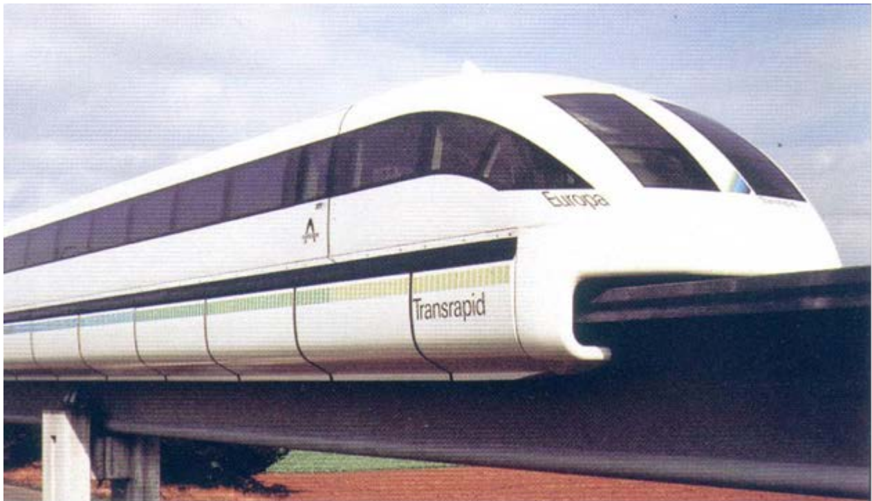
Fig. 5: The 1992 Transrapid 07 with long-stator linear motor, 90 t, 450 kmph. Test track 31.4 km.
