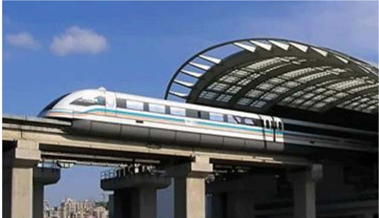
Fig. 6: The 2002 Shanghai MAGLEV Transportation with long-stator linear motor, 505 kmph. Track 30 km.
