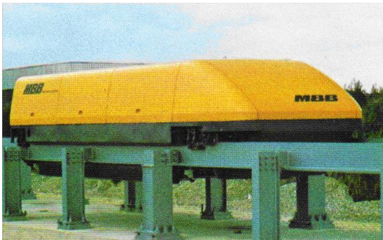
Fig. 2: The 1975 MBB Komet with rocket engine, 8.8 t, 401.3 kmph. Double-span steel test track 1.3 km.
