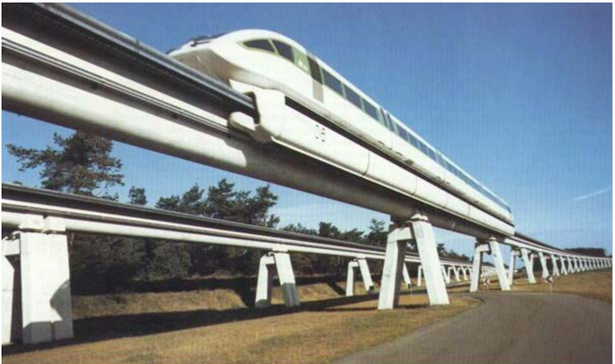
Fig. 4: The 1982 Transrapid 06 with long-stator linear motor, 120 t, 412 kmph, 200 passengers. Track 31.4 km.
