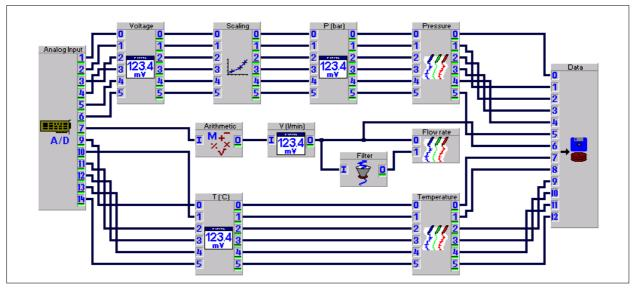
Fig. 6 Block diagram of the measurement system
