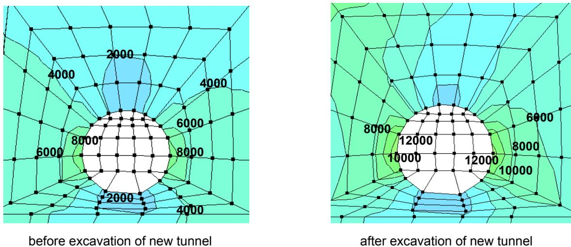
Fig. 6: Contour lines of vertical stresses around water transmission tunnel
