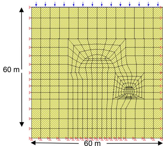
Fig. 5: FEM-mesh, boundary conditions, contours of underground openings
