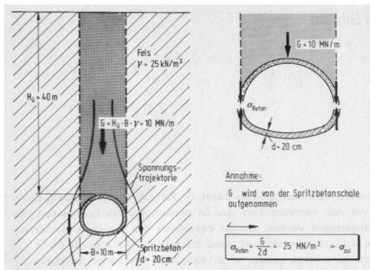
Figure 3: Stress diversion around a tunnel with a width of 10 m sealed by 20 cm shotcrete
