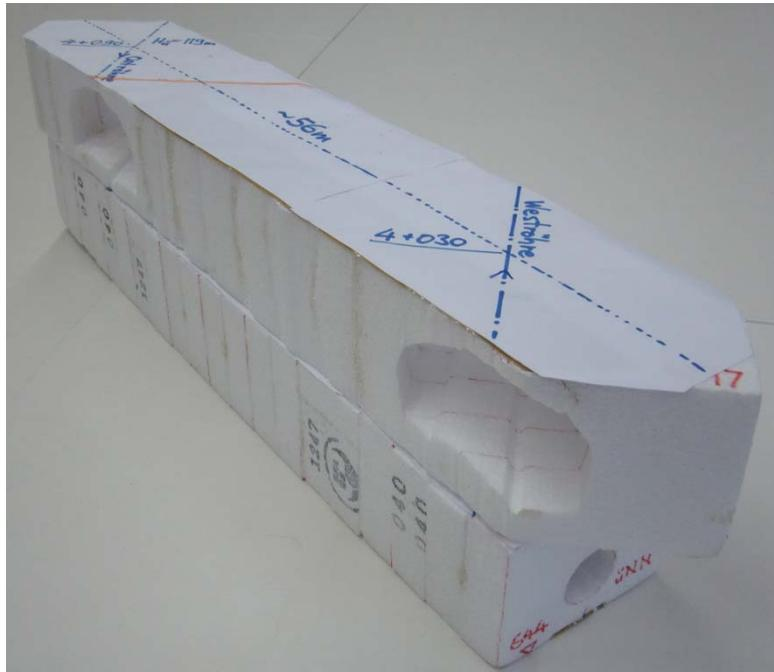
Figure 2: 3-D model of tunnel intersections
