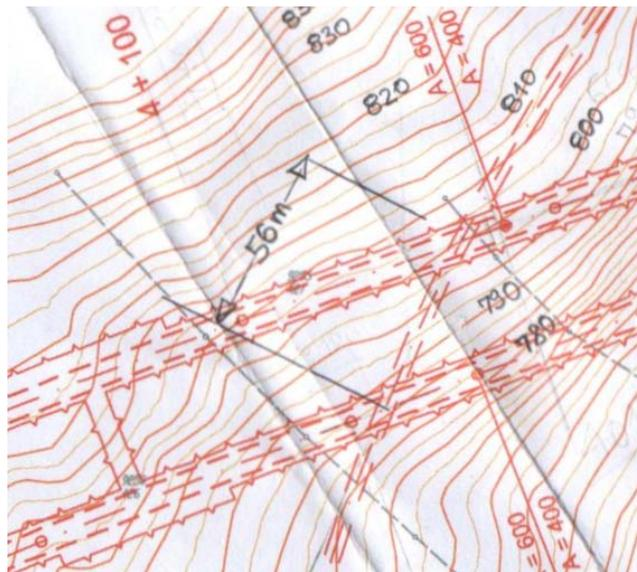
Figure 1: Topographic contour line map with existing tunnel and twin-tube tunnel
