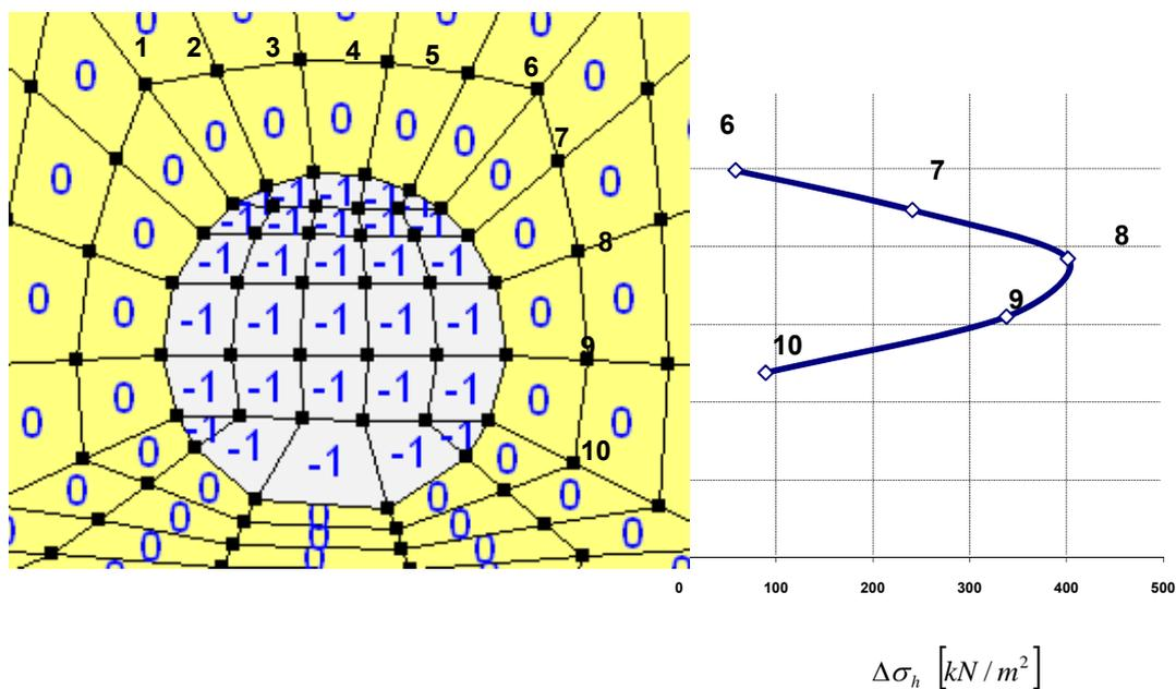
Fig. 7: Additional stresses in the circumference of old tunnel due to excavation of highway tunnel
