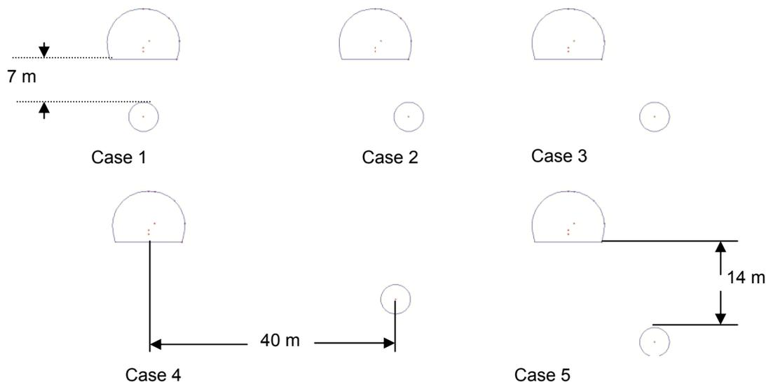
Figure 4: Investigated geometric relations (Case 1 – 5) between underground openings
