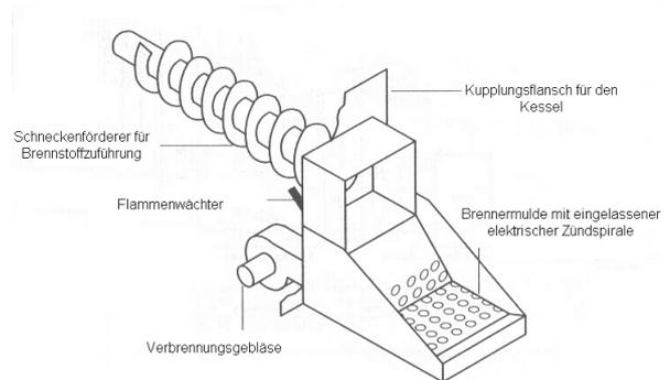
Fig. 2: Screw-conveyor
