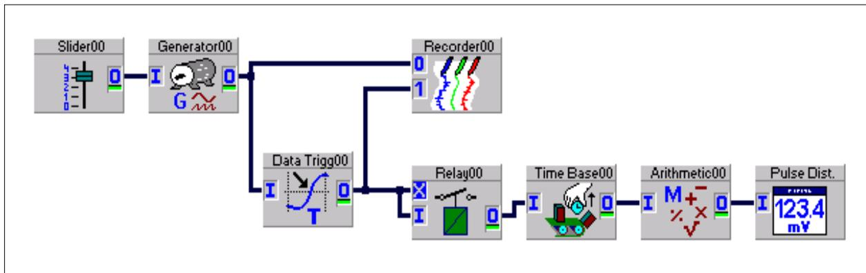
Fig.2 Calculation of pulse distances
