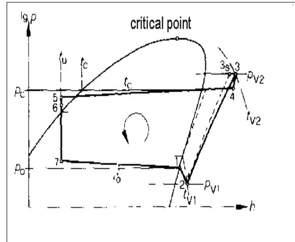
Fig. 4 Lg p/h-diagram of the refrigerant
