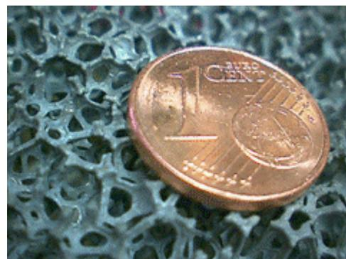
Figure 5: 10ppi metal foam as compared to a one Euro cent coin
