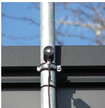
Abb. A8 Pyranometer horizontal (THN-AR)
