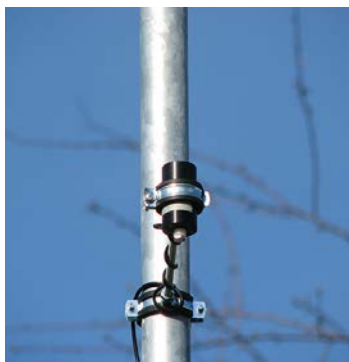
Abb. A9 Pyranometer vertikal (THN-AR)
