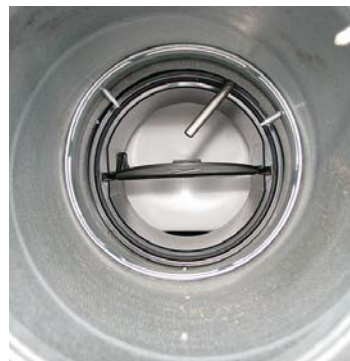
Abb. A13 Ansaugtemperatursensor DFL (THN-AR)
