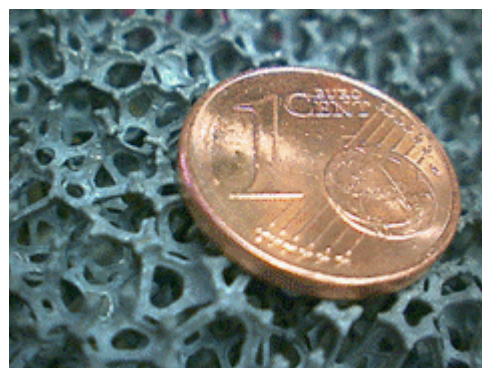
Figure 5: 10ppi metal foam as compared to a one Euro cent coin
