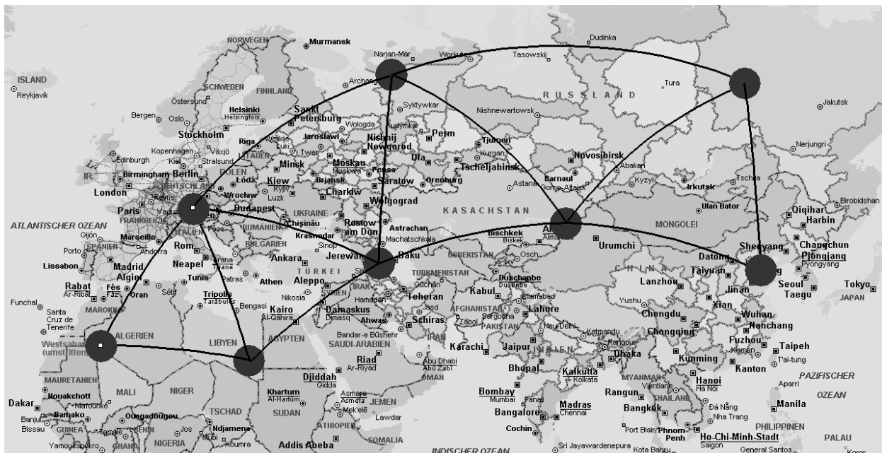
Fig. 15: Example of areas with diameters of 400 km each (dark spots) where the same channel in the 26 MHz could be used. The spacing between these areas is 2900 km to guarantee a minimum distance of 2500 km between co-channel transmitters which the predictions suggest is sufficient to avoid mutual interference.
