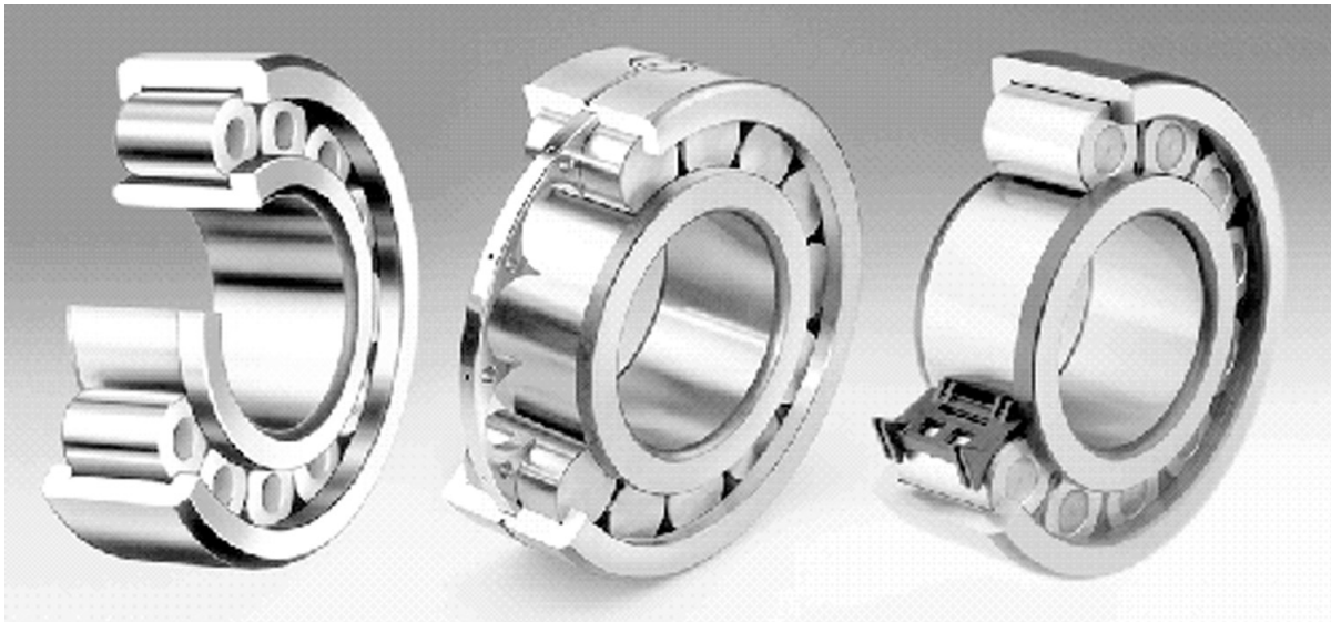
a) b) c) Fig. 1: INA Cylindrical Roller Bearings series a) SL 1923, full complement radial cylindrical roller bearing b) LSL 1923, radial cylindrical roller bearing with a brass disc cage c) ZSL 1923, radial cylindrical roller bearing with plastic spacers
